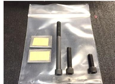
The shims have a strip of double stick tape on one side. Peel the tape and stick the shim to the clamp as shown in the photo above. If you need to add the second shim, stick it to the back of the first shim. (Note: removing the floating half round makes this process easier. It is just held in with a magnet.) Be sure to install the shims all the way down in the pocket and not sticking up above the clamp.
